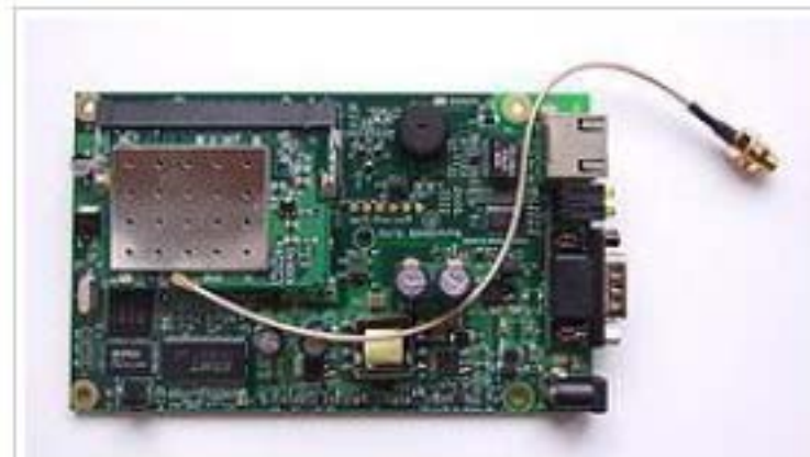
An embedded RouterBoard 112 with U.FL-RSMA pigtail and R52 miniPCI Wi-Fi card widely used by wireless Internet service providers (WISPs) in the Czech Republic.
